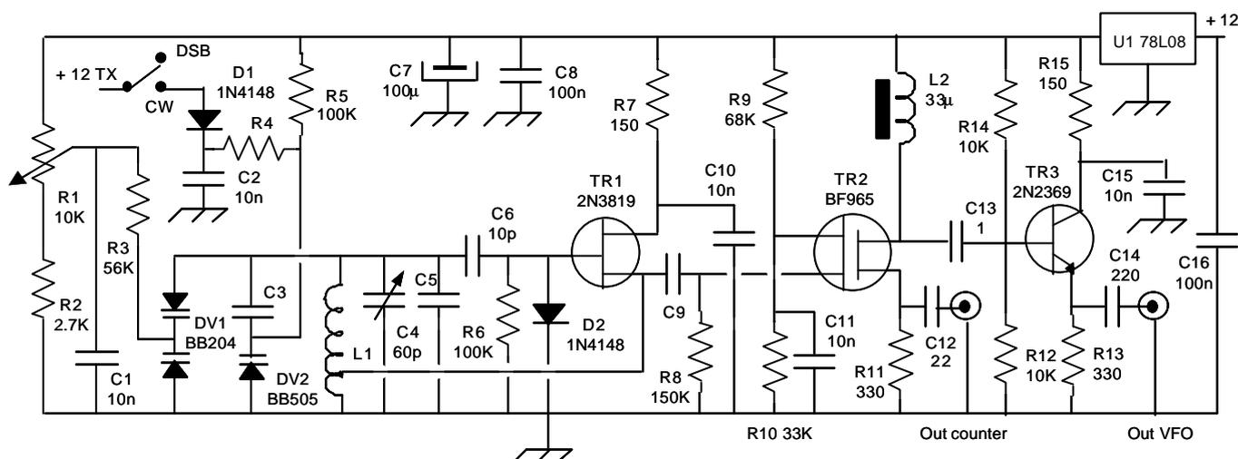
Dealing with a direct conversion circuit, the VFO and the transmitter work on the same frequency, therefore some care must be taken to avoid interference between the two stages. I suggest to put the VFO board into a little tin-plate box (better than aluminium), avoiding to mount it too near the final TX stage.
