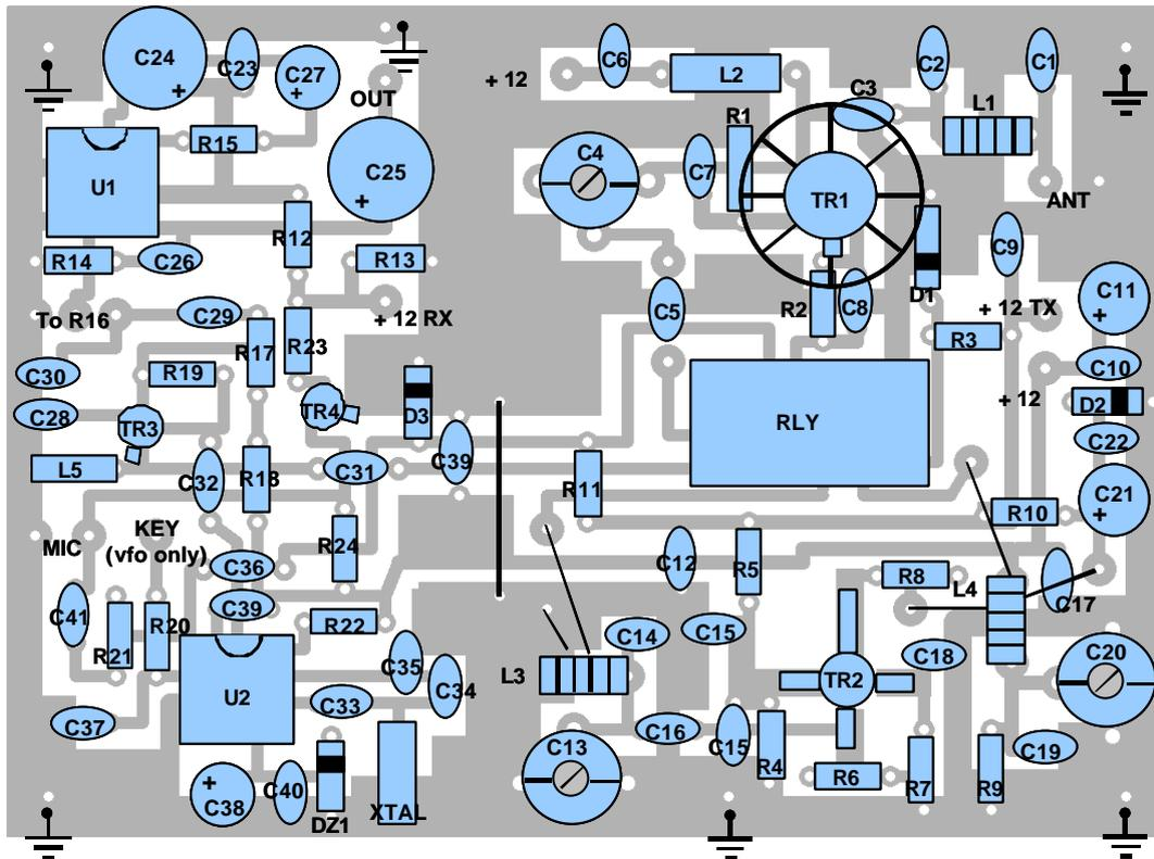
The whole circuit must be put into a metallic box to avoid humming and microphonic effect, common in direct conversion devices, for the same reason the grounding of the PCB must be effective, as shown in the drawing. Note that the TX final stage supply is kept apart from the rest of the circuit, so reducing possible RF feedback and consequent instability, for the same reason the preselector toroids are rotated 90 degrees. The rig may be set up in the following manner :
